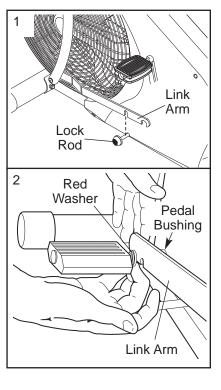
gers as shown. **Be careful not to pinch your fingers.** Next, slide the link arms onto the pedal bushings. Move the link arms up and down slightly to make sure that they are fully seated on the pedal bushings. **CAUTION:** Make sure that the link arms are fully seated on the pedal bushings. If the link arms are not on the pedal bushings, they may slip off during use, resulting in injury to the user.
